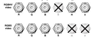
Figure 5 — Output connections
